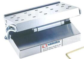
Design by the principles of SINE, angle grinding can be done well. High precision of parallelism within 0.002mm and squareness within 0.005 mm. Setu, and dressing time reduced to a bare minimum due to simplicity.(ANGLE 0° - 46°)
